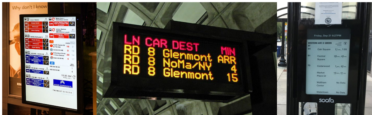
Figure 6. From left: examples of LCD, LED, and E ink transit screens in use.
