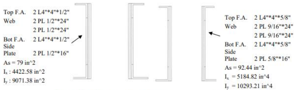
(f). Typical section; Node L2-L3, L5-L6 (Bottom Chord)
