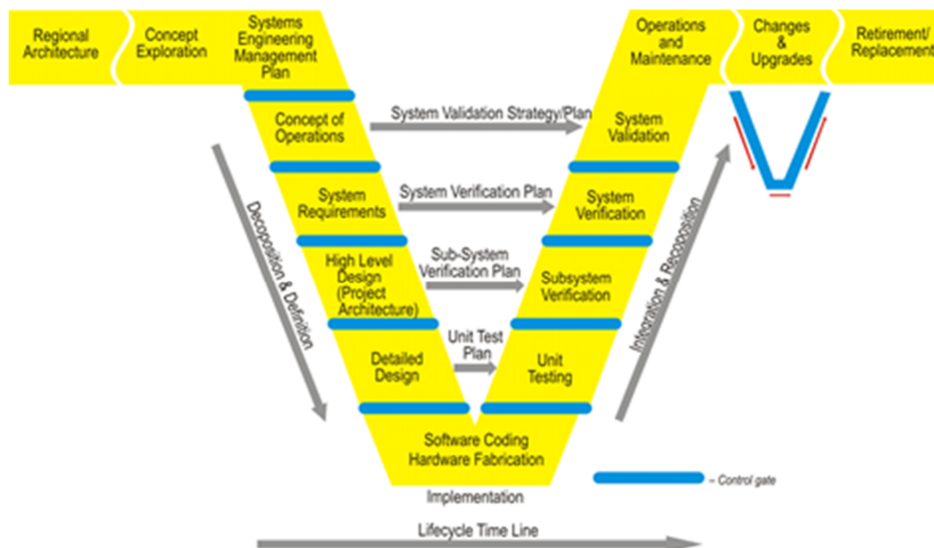
Figure 3 – Systems Engineering "V" Diagram
