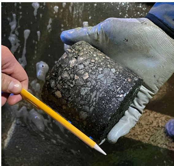
Figure 13: Picture of core immediately after being exhumed
