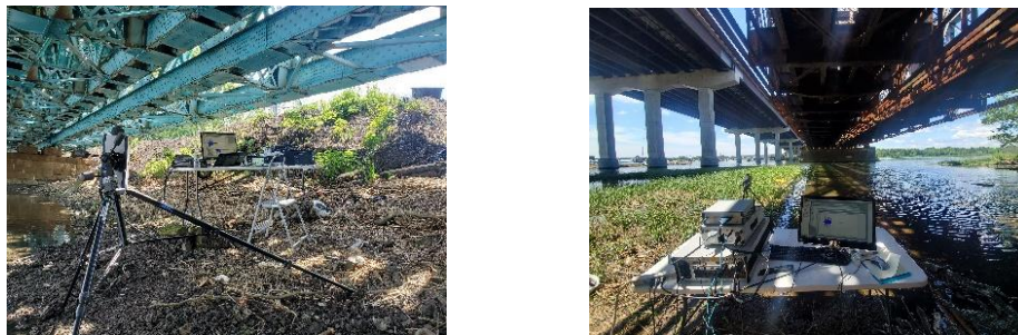
Figure 15 - LDV setup during field tests: (left) Cos Cob Bridge and (right) Devon Bridge
