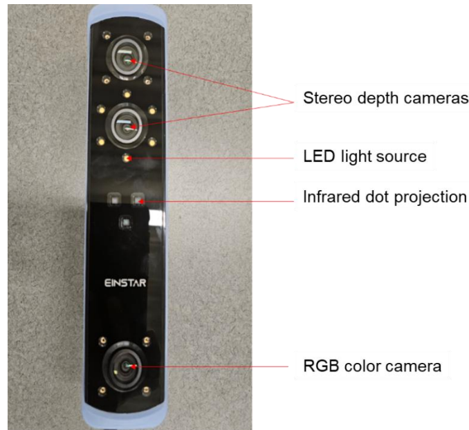
Figure G-2 Structured Light 3D scanner.
