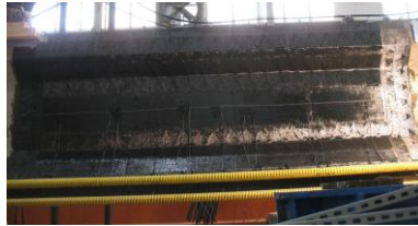
(b) I-3 with a complete wrap in the vertical direction and sheets in the horizontal direction.
