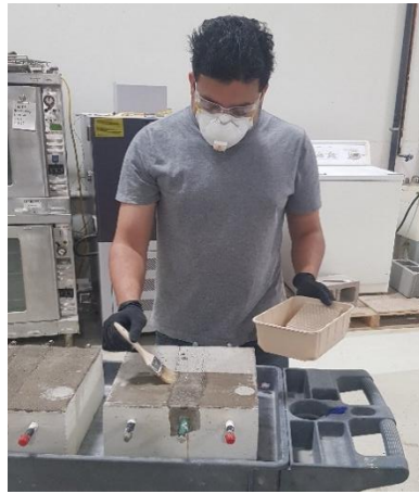
(a) Silane penetrating sealer application
