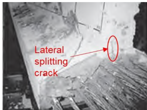
Figure 4-16. Lateral splitting cracks documented at the BT-63a beam end (Hawkins and Kuchma 2007).
