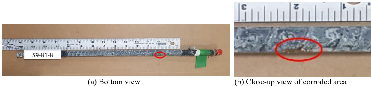
Figure 5-17. Condition of Rebar-1 from S9 specimen.
