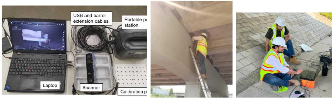
(a) (b) (c) Figure G-4 (a) Scanner, laptop, and other accessories, (b) scanning a beam end, (c) checking data during scanning.
