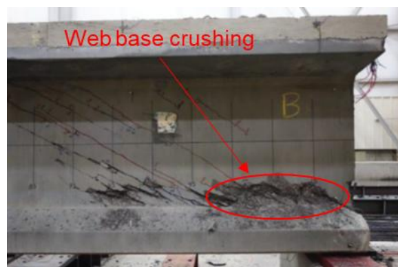
Figure 4-18. Failure patterns of BT-54b specimen (Shahrooz et al. 2017).
