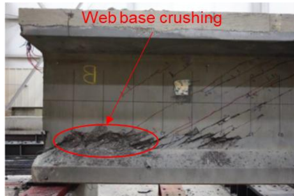
Figure 4-10. Web base crushing failure of a bulb tee section (Shahrooz et al. 2017).
