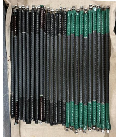
(c) Rebars with shrink tubes at both ends
