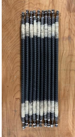
(b) Electroplater tape wrapping at both ends
