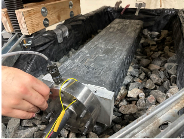
Figure 41. Wear on HDPE Crosstie.
