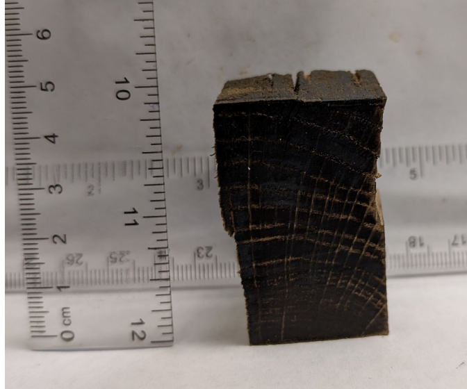
Figure 7. Photos of Cross-Grain Wood Testing Specimens.
