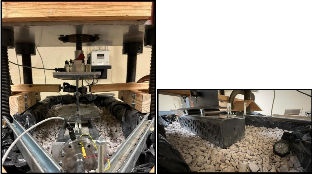
Figure 34. Photos of Friction Test Set-Up.
