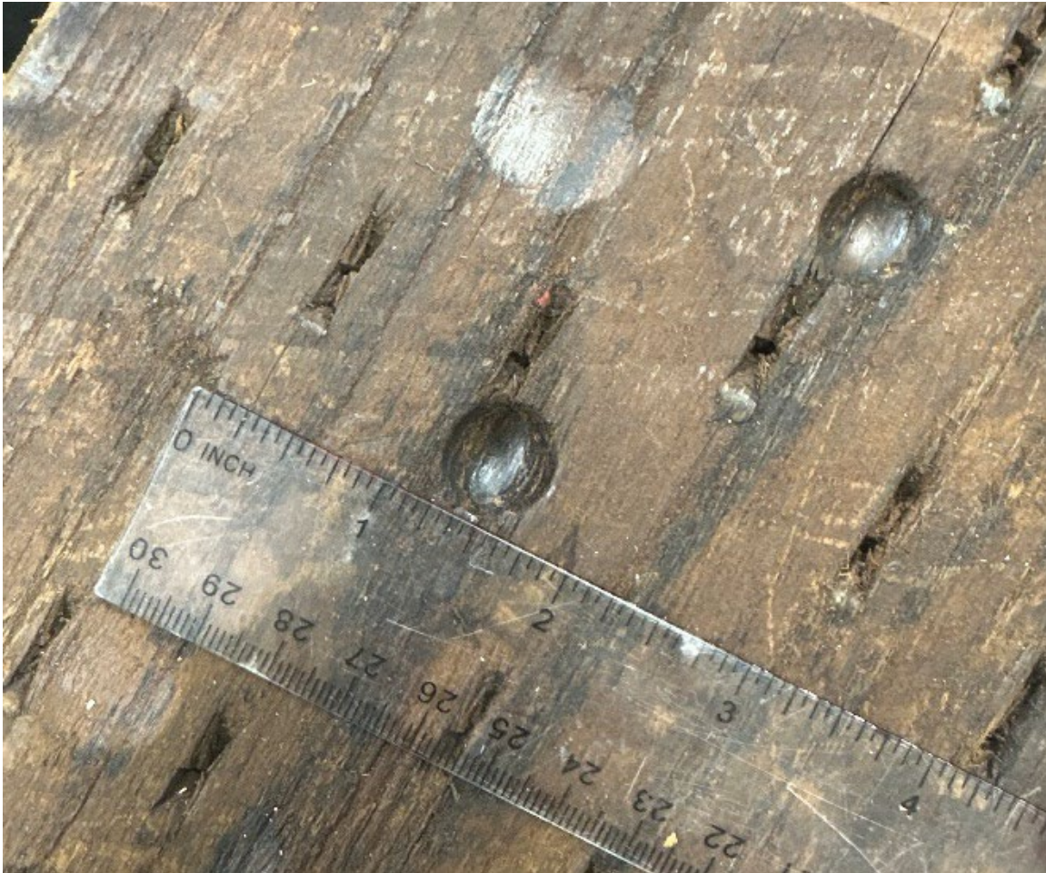
Figure 13. Post-Test Indentation from 15 mm Ball on Dry Wooden Tie.
