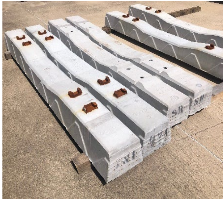
Figure 39. Concrete Crosstie at Texas A&M for Testing.
