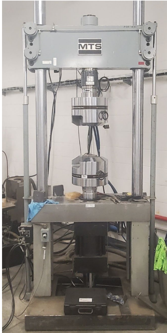
Figure 7: The 100 Kip MTS Machine Utilized for the Cyclic Fatigue Testing of the Railhead
