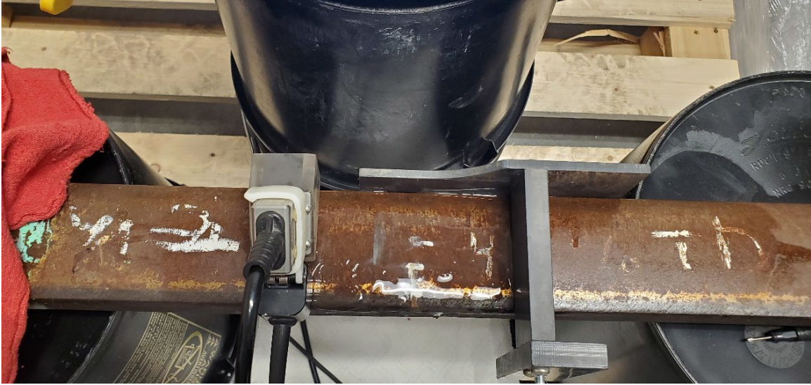
Figure 8: Photograph of Test Specimen Periodically Interrogated with a Phased Array to Assess Internal Crack Growth Due to Cyclic Uniaxial Loading
