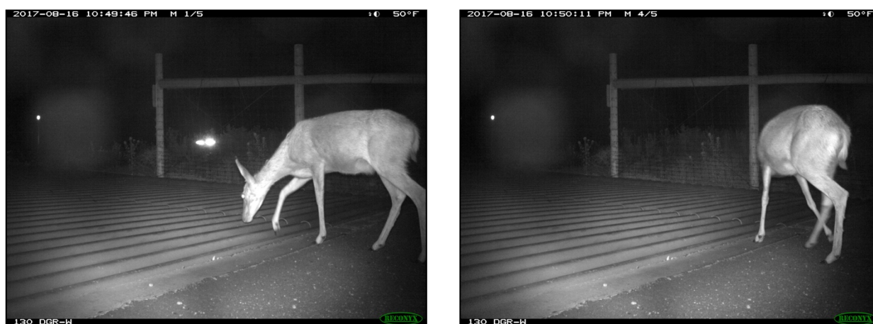
Figure 29. Mule deer approaching and ultimately repelling from the round deer guard at County Road 1002.
