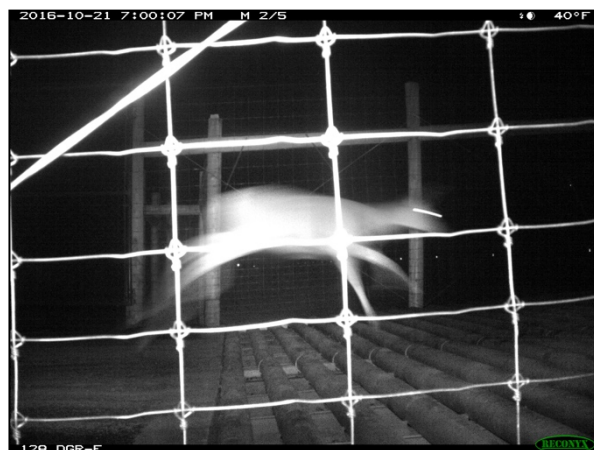
Figure 30. Mule deer jumping across the Triangle Road round bar deer guard.
