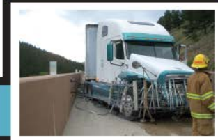
Used CatchNET August 26, 2010. No injuries, minimal damage. 15,000 lbs, 60 mph, used 1 net.
