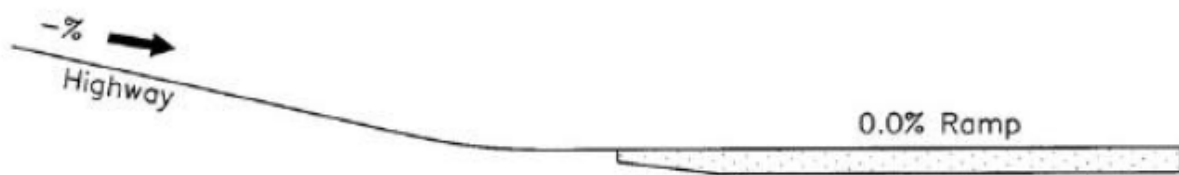
Figure 1.5. Horizontal Grade EER Reprinted from AASHTO’s Green Book (p. 144), by the American Association of State Highway and Transportation Officials, 2011, Washington DC.
