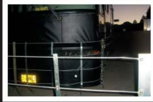
Used CatchNET May 29, 2012. No injuries, minimal damage. 55,000 lbs, 70 mph, used 7 nets.
