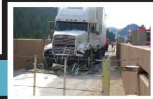
Used CatchNET August 26, 2010. No injuries, minimal damage. 15,000 lbs, 60 mph, used 1 net.
