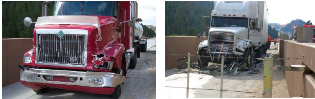
Figure 1.12. Wyoming Dragnet EER Crash Damage Reprinted from Wyoming Department of Transportation. Retrieved June 15, 2017, from https://www.wyoroad.info/Highway/RunawayTruckRampInfo2013.pdf , Copyright Wyoming Department of Transportation, 2013.
