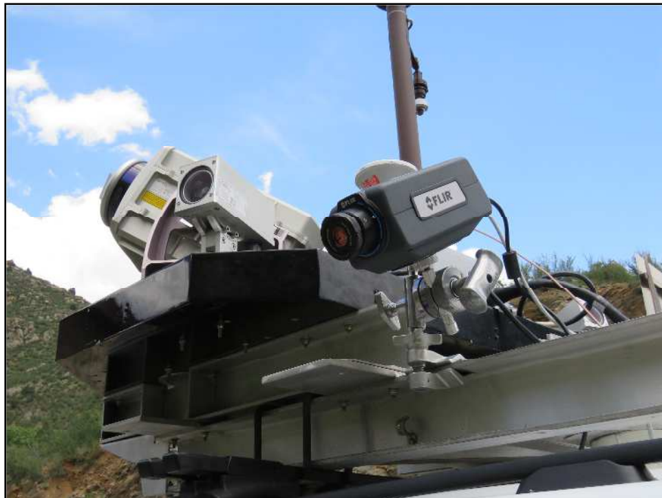
Figure 8: FLIR A6750 mounted to SAM mobile truck
