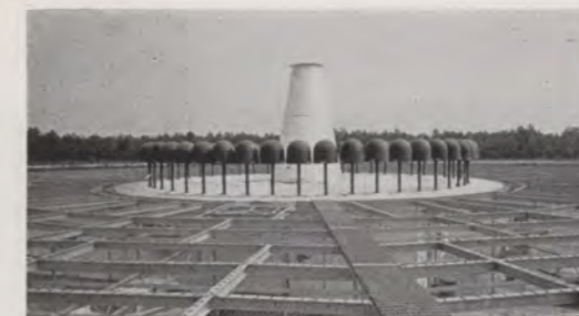
Doppler VOR advanced navigation equipment tested at NAFEC provides improved signals for aircraft guidance.
