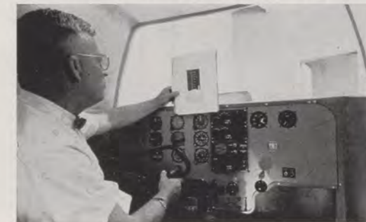
Designs for simplified cockpit for light aircraft—Project Little Guy—will be studied in this simulator.
