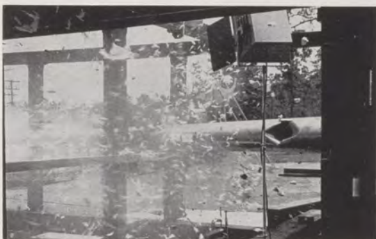
Major program at National Aviation Facilities Experimental Center concerns problem of bird strikes on aircraft, the ingestion of birds into aircraft engines. Two major accidents, several lesser incidents, have been caused by birds in recent years. "Bird gun" facility, in which dead birds, foreign objects including ice pellets are fired at aircraft components, continually examines problem. Here dead chicken is weighed, loaded into "gun," fired at aircraft tail section.
