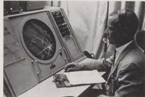
Flight-operation studies including airport approach, departure and pilot reaction in collision avoidance are conducted in F-100A flight simulator at right. Below, evaluating traffic control radar bright display.
