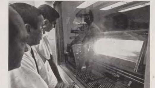
Fire Test Cell and Blower Facility is used to study fires in aircraft engines, components. Above, external view. Below, technicians observe from control area.
