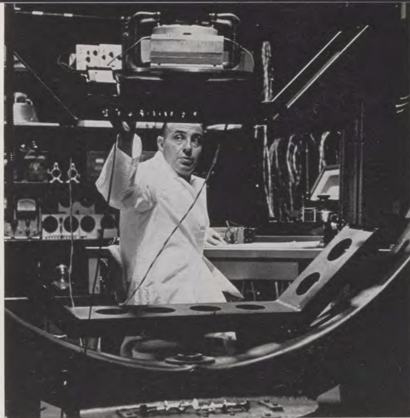
NAFEC has outstanding record in field of airport lighting. Below, engineer adjusts lights on test visual approach indicator. Right, checking "pancake" light for even intensity.
