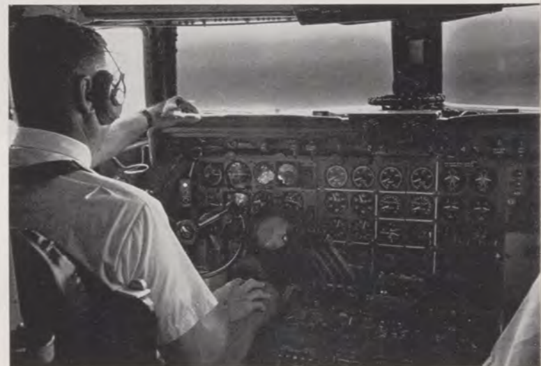
More than 1100 successful "hands-off" landings have been made in FAA DC-7 aircraft fitted with developmental automatic all-weather landing system. Above, automatic approach. Below, checking gear.
