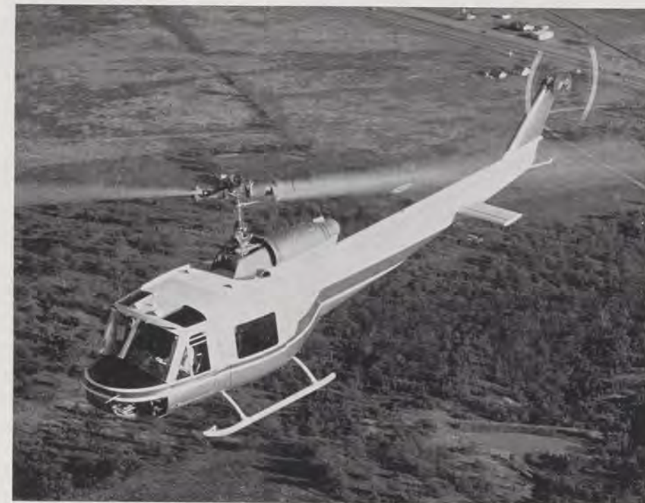
FAA's Certificate of Airworthiness was given last month to this Bell 204B helicopter, a commercial version of the U. S. Army's battle-tested UH-1B Iroquois. The 10-place helicopter has a gross weight of 8,500 lbs., can carry a useful load of 3,900 lbs. Cruising range is 230 miles at 120-138 mph.
