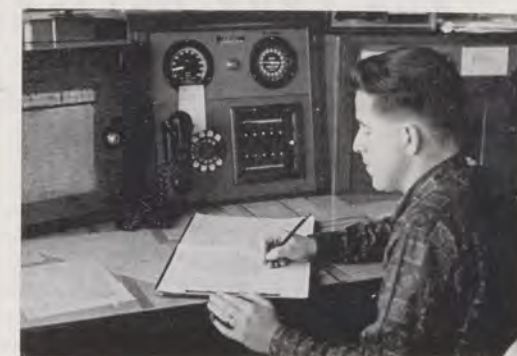
Above, weather observer checks ceilometer which measures height of cloud bases with photo-electric cell that scans sky. He can also obtain the information, plus other data, from remote console (right).
