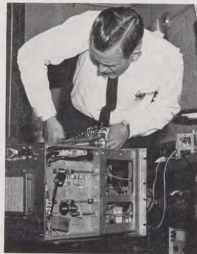
Left, on the "bedsprings" antenna of fan marker, FAA technician records current. Remote UHF transmitter above, and receiver in airport control tower below, get overhaul to keep them in top operation condition.
