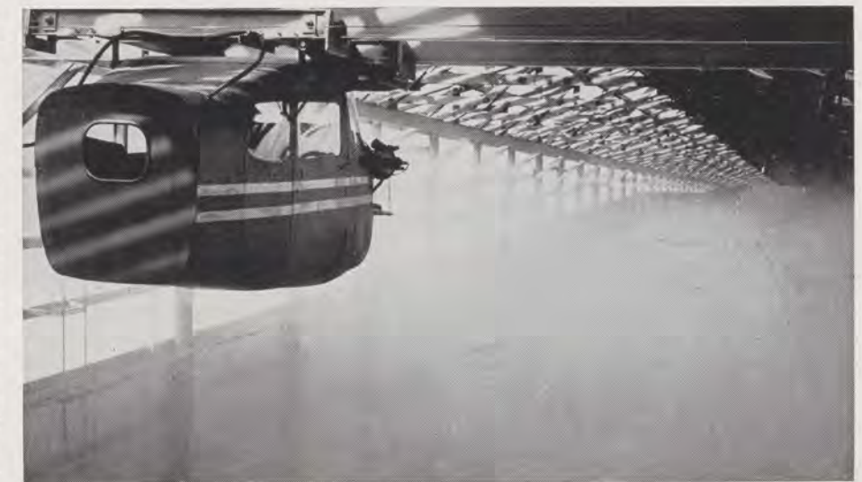
Fog chamber for testing runway lights under low visibility is 800 feet long, 30 feet wide. Picture below was taken before fog had built up to uniform density. Approach and runway lights, dimly seen, are on.
