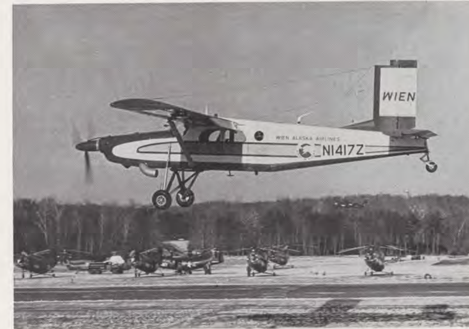
First single-engine turbine airplane type-certificated by FAA, the Pilatus Turboporter, was built in Switzerland. Eight-place airplane cruises at 137 mph, has maximum operating altitude of 25,000 ft.
