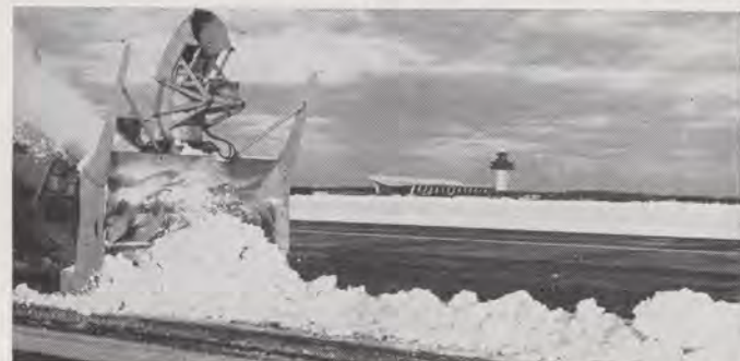
Close-up rotary snow blower (above) shows auger in front. Below, snow plow with roll-over blade is versatile machine. Photos by Reynolds & Co.
