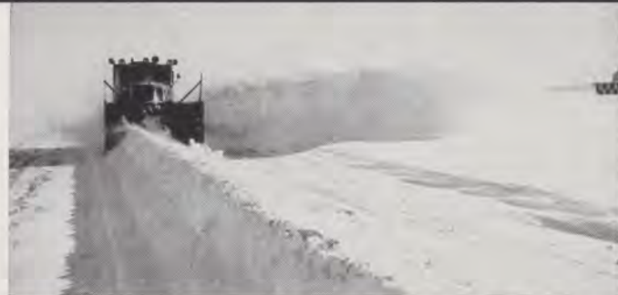
Efficient rotary snow blower chews up snow, blows it up to 150 feet away.
