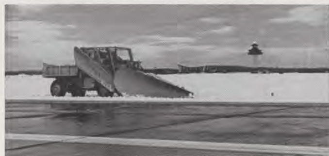
Close-up rotary snow blower (above) shows auger in front. Below, snow plow with roll-over blade is versatile machine. Photos by Reynolds & Co.
