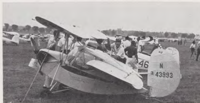
Mignet Flying Flea with 40-hp Continental engine, built by Frank Easton of Salem, Ohio, has unusual tail with horizontal stabilizer set forward.
