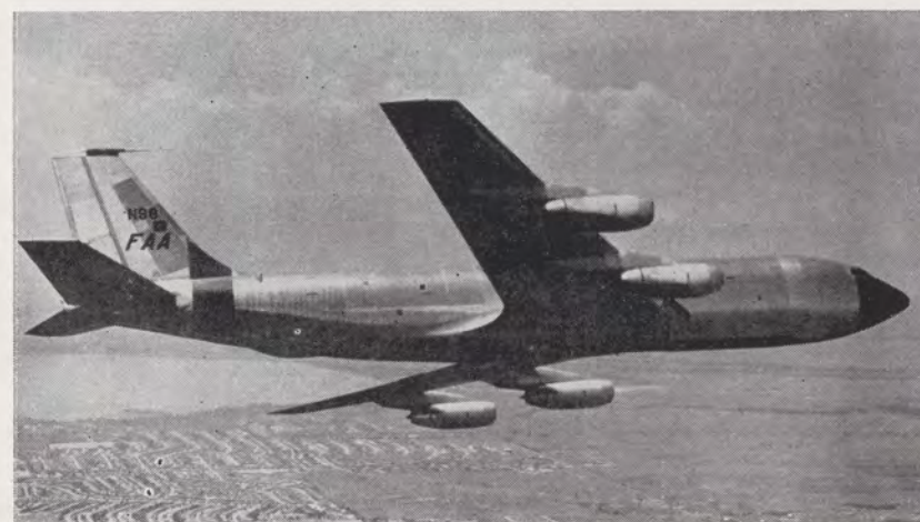
Boeing C-135 for high altitude (above 25,000 feet) flight checking of nav aids.
