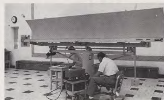
Calibration crew at test mount carefully plots patterns of recently overhauled antenna array used on a Precision Approach Radar.
