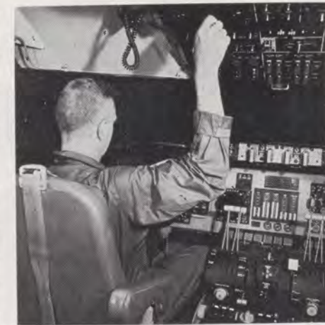
Close-up of the C-141A Starlifter cockpit showing control panel and proposed new taped instruments.
