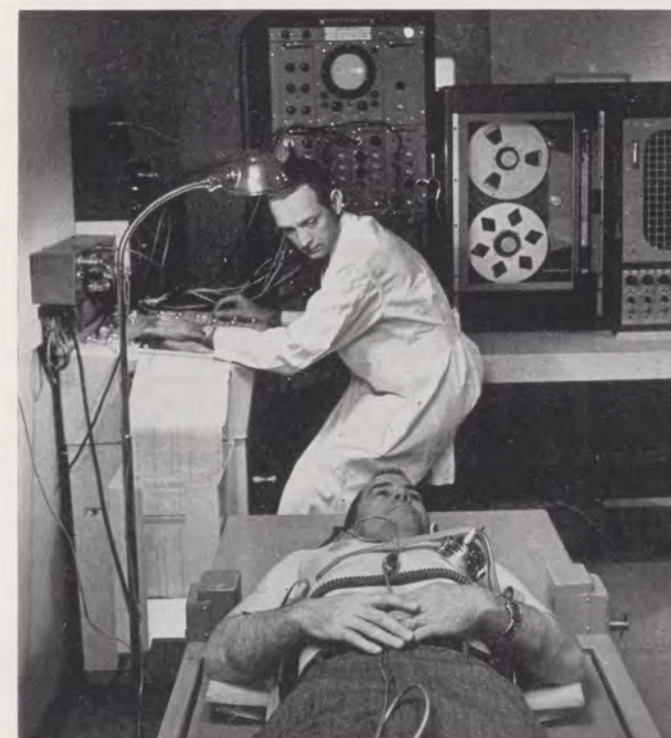
On ballistocardiograph, a vibrationless "bed" suspended to minimize gravity, microphones measure heart which normally vibrates 5/1,000 of an inch.
