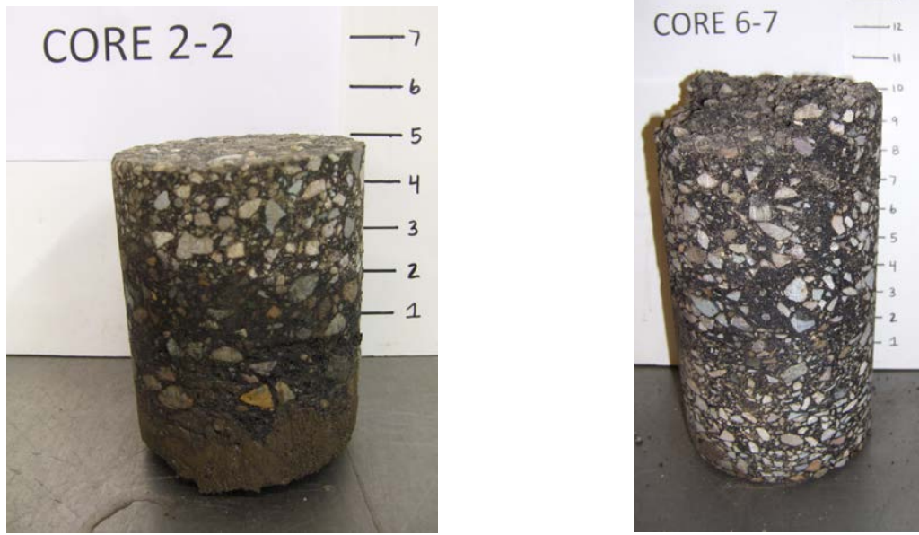
Figure 7. Examples of dry (site 2) and emulsion-stabilized FDR (site 6) cored samples
