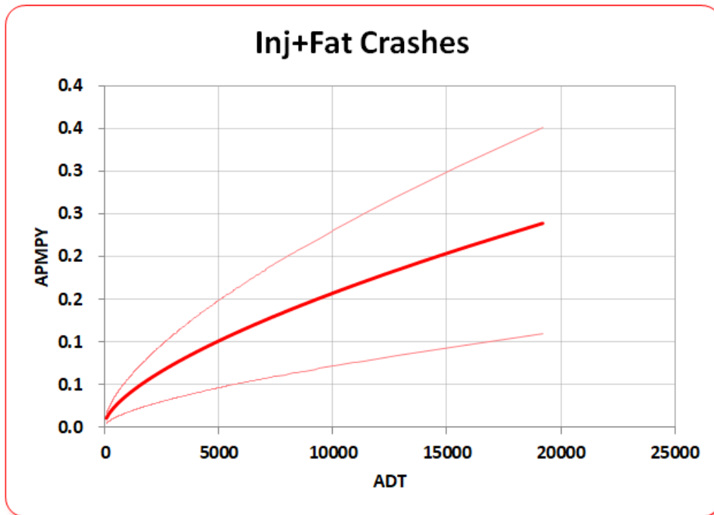
Figure 78. SPF - Rural Flat and Rolling 2-Lane Highways – Wild Animal Collisions – Severity Model
