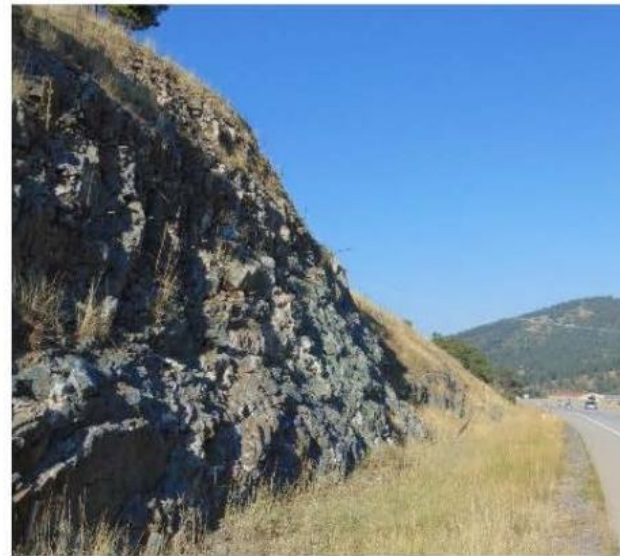
Schistose texture of intact rock
