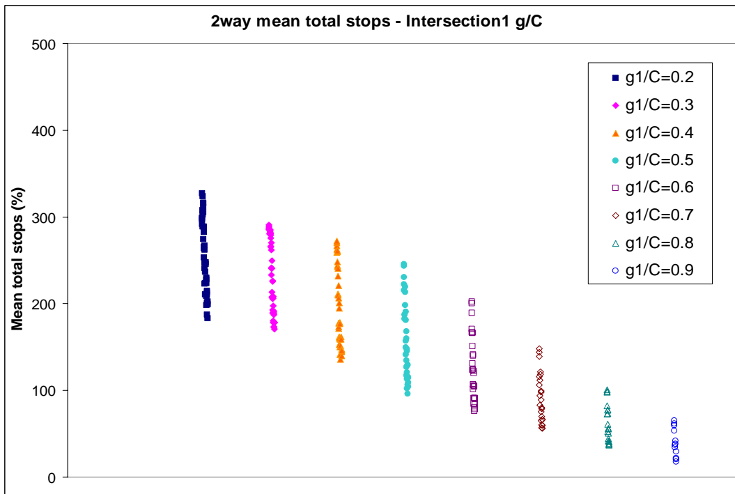
Figure 13. G1/C Effect on Two-Way Intersection Stops.
