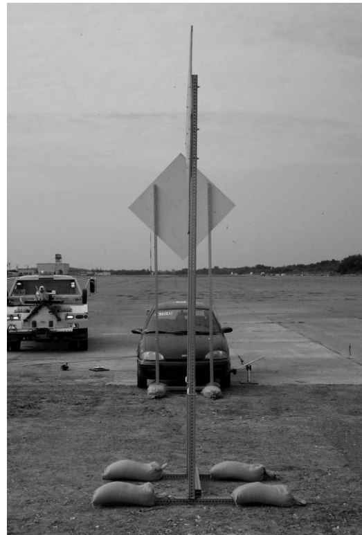
Figure 5-2. Vehicle and Support Geometrics before Test.
