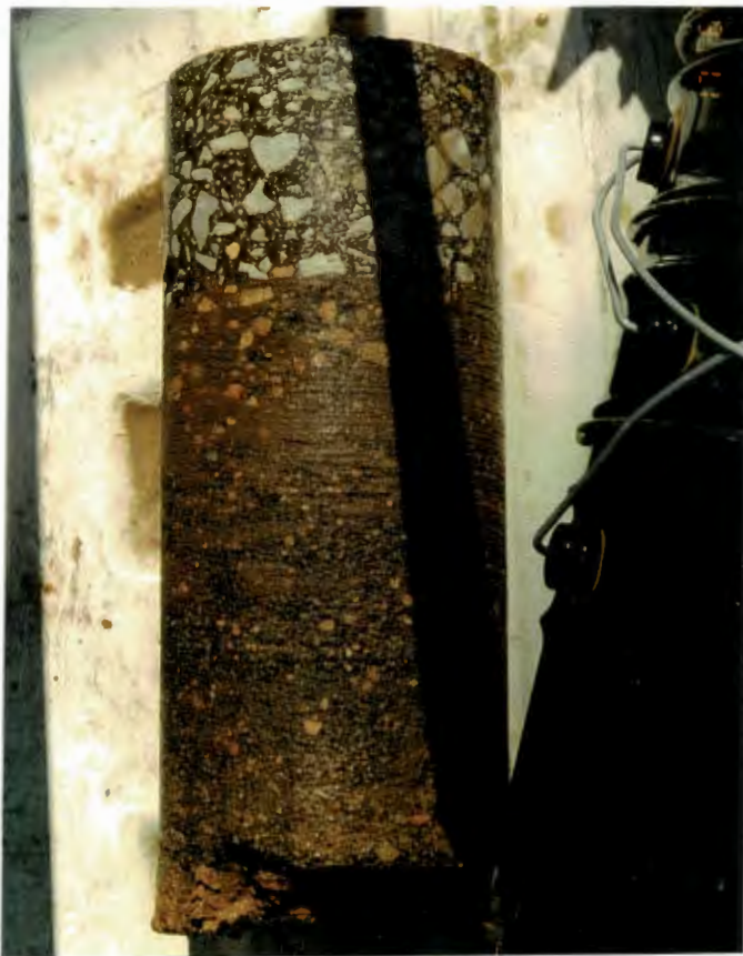
Photo 2. Core Representing Existing Layer Thicknesses
