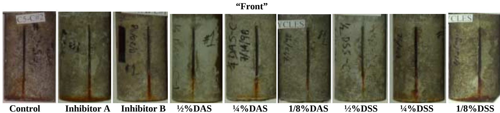
Figure 5.33 Final exterior appearance of the oven-dried pre-cracked specimens. Only the “front” side is shown because this is where the corrosion was induced.
