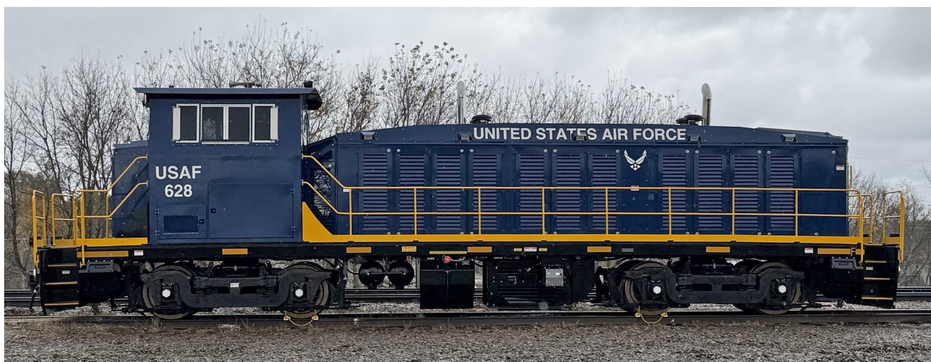
A recent U.S. Air Force locomotive fully assembled and moved to the tracks for testing. After successful testing by the vendor in Minnesota, the locomotive was delivered to USAF Joint Base Charleston. Source: U.S. Air Force.
