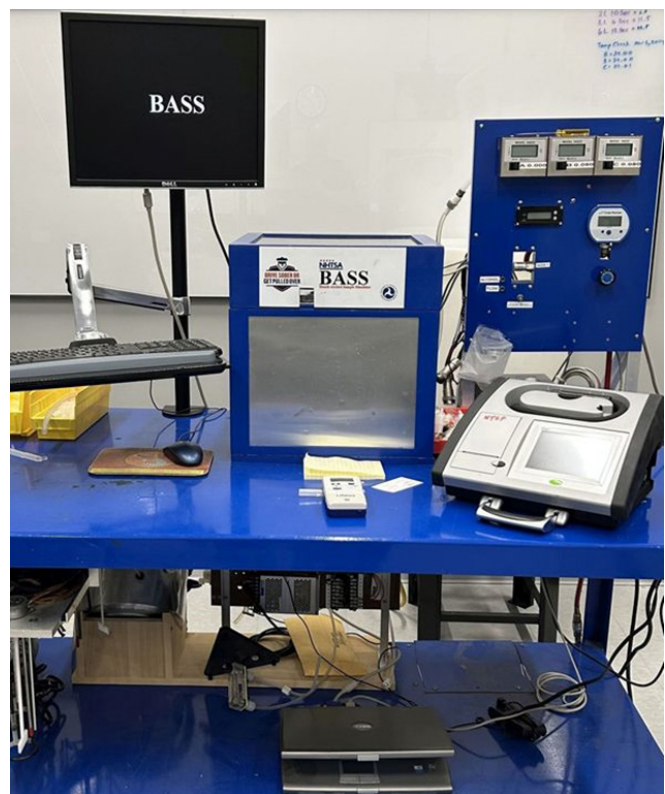
The U.S. DOT Volpe Center's BASS Drinking Driver Robot, which is used to simulate breath samples from impaired drivers. Source: U.S. DOT Volpe Center.
