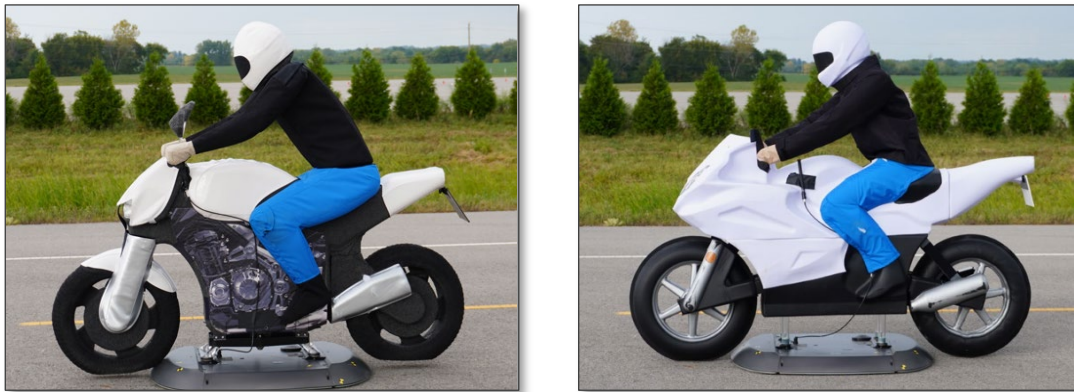
Figure 3. The 4a 4activeMC-EMT (left) and ABD Soft Motorcycle 360 (right), each secured to an ABD LaunchPad 80 robotic platform
