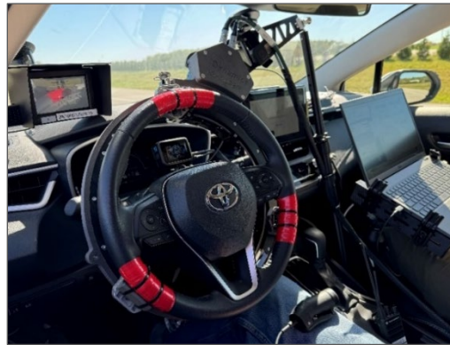
Figure 4. Robotic steering controller installed in an SV
