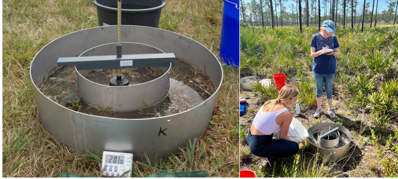
Figure 4.3. Collection of field infiltration data.
