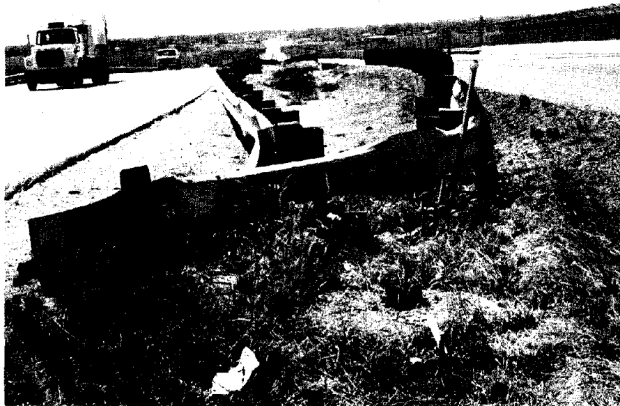
FIGURE 35: Impacting vehicle was safely decelerated without vaulting the guardrail.
