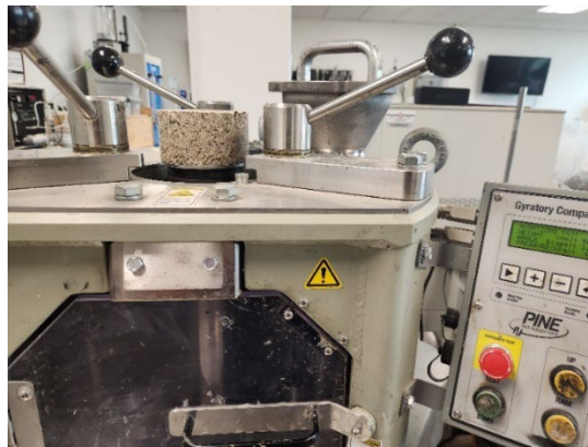
(a) A fabricated sample using SGC
