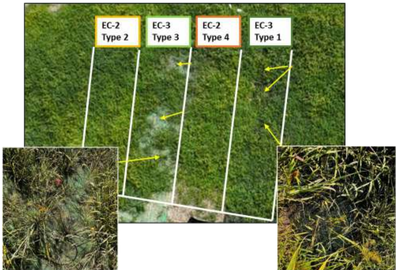
Figure 13. Rolled Erosion Control Product Plots at the Richmond Site, Week 9 (top) and Waynesboro B site, Week 16 (bottom). The plots illustrate the visible bare patches of the light green EC-3 Type 3 mat and the dark green EC-3 Type 1 mat. Bare patches on the dark green EC-3 Type 1 mat are difficult to see in the upper image; large areas of sparse vegetation are indicated by arrows.
