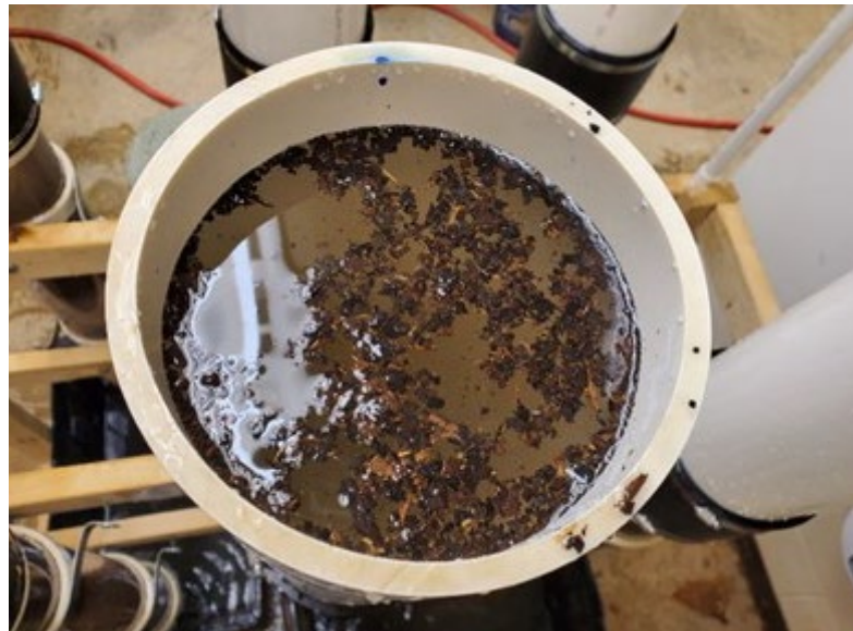
Figure 2.14. Pine Bark Fines Floating During Tests on F3 Designs.
