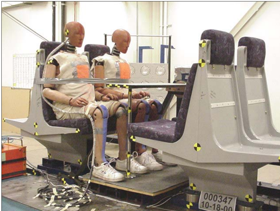
Figure 19. Pre-test Photo of Test No. 2, Baseline with Table
