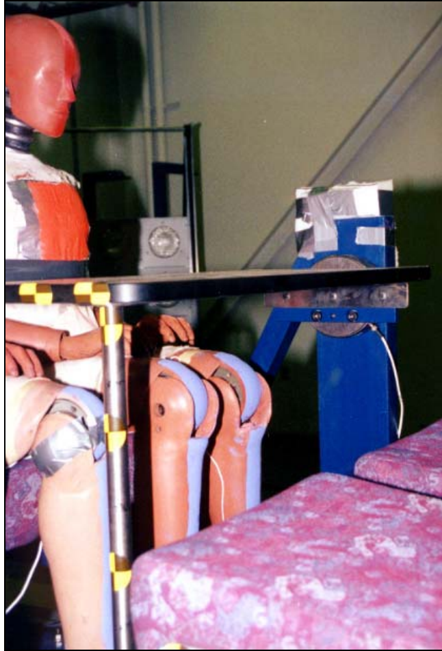
Figure 20. Pre-test Photo of Test No. 2, Focusing on the Table Attachment
