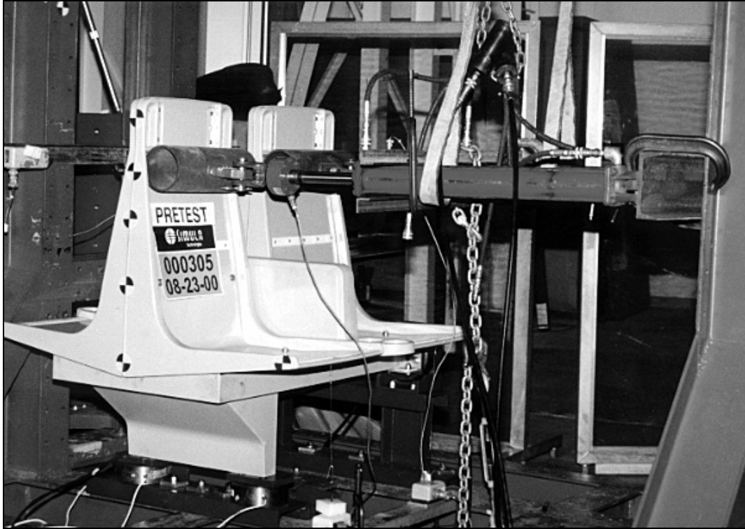
Figure 5. Seat Static Test - Pre-test Photo of Seat System and Test Equipment
