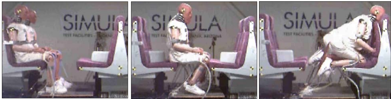
Figure 24. Test No. 3, Occupant Kinematic Sequence for Two 50th-percentile ATDs, 9 G Peak Acceleration
