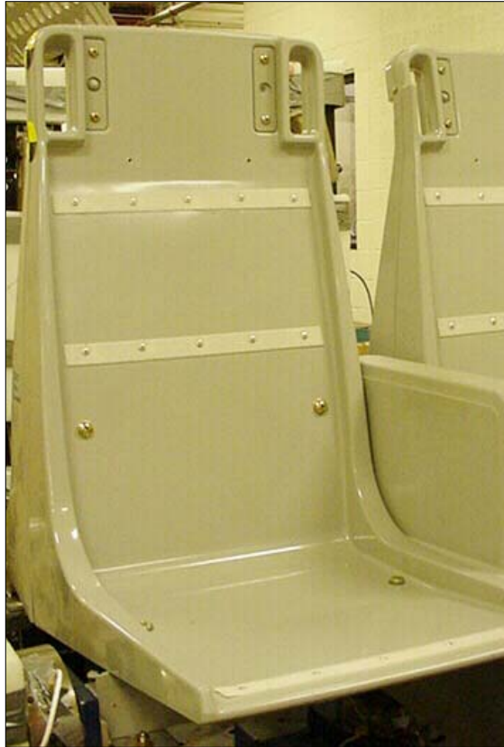
Figure 2. Thermoplastic Seat Pan/Back Structure
