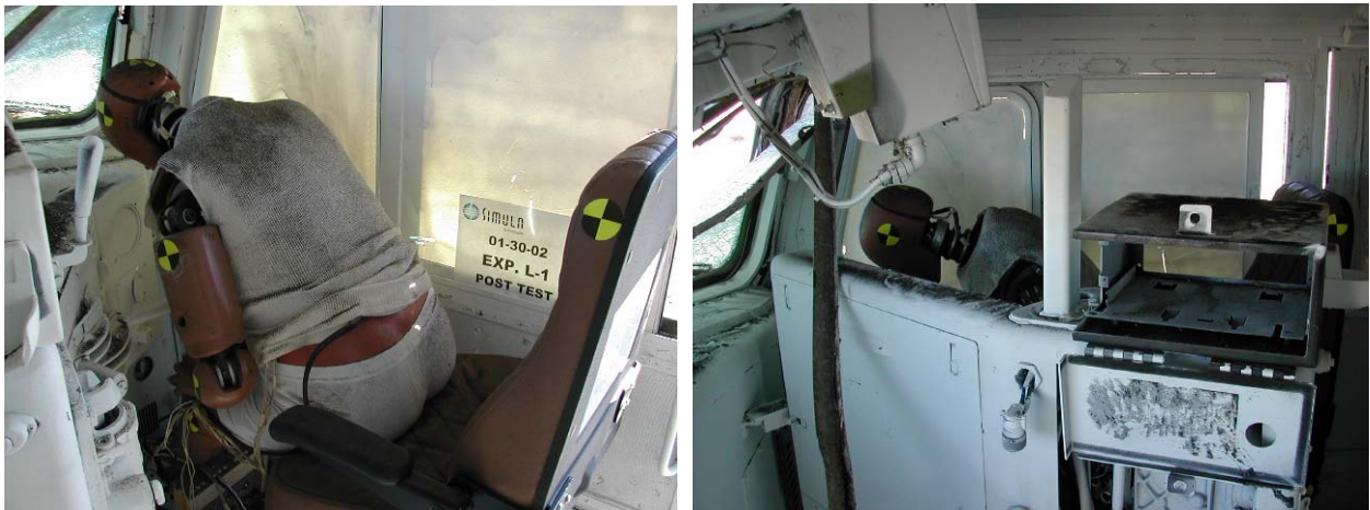
Figure 43. Experiment No. L-1 - Post-Test View of the ATD in the Operator Seat
