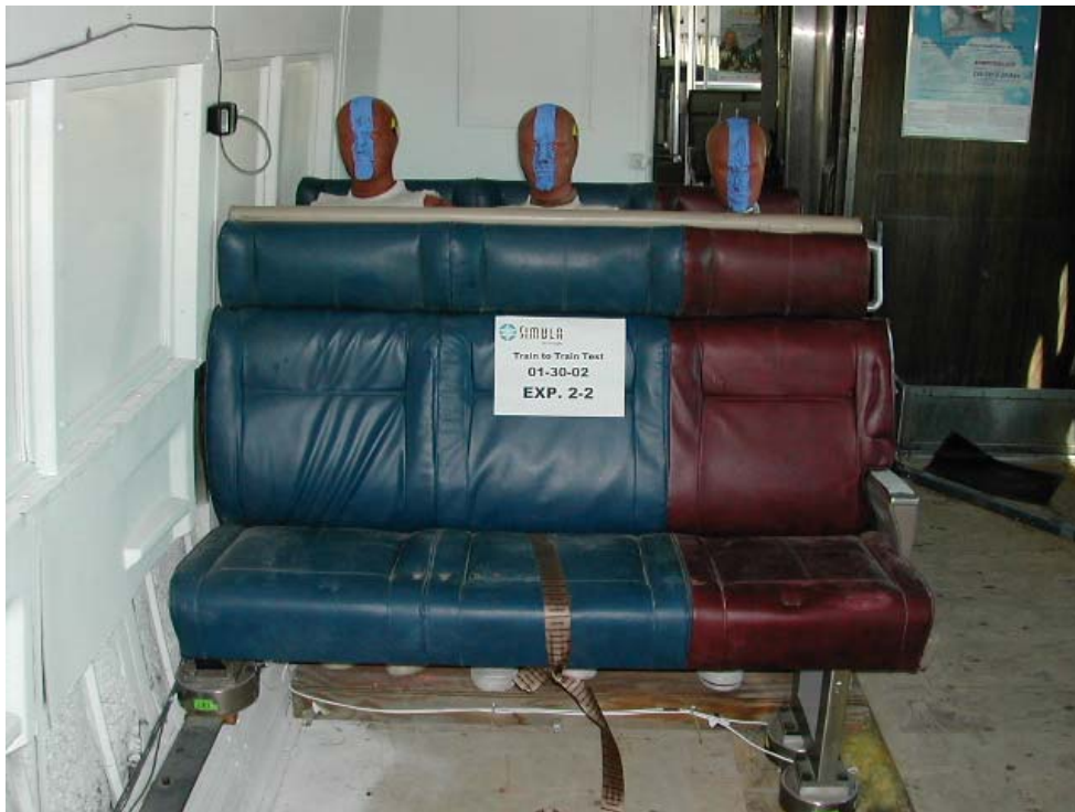
Figure 20. Pre-Test Photo of Experiment No. 2-2, Row-to-Row M-Style Seats
