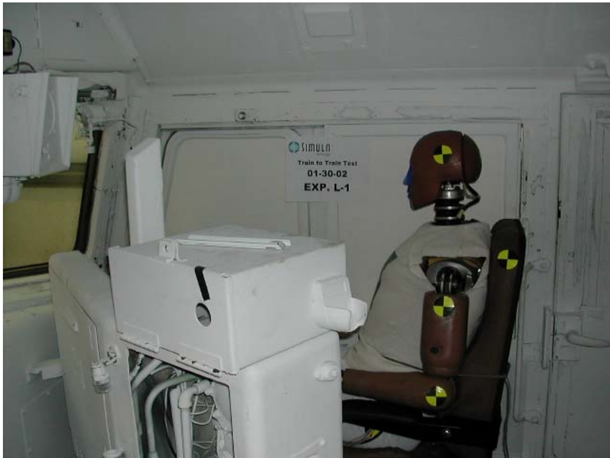
Figure 21. Pre-Test Photo of Experiment No. L-1, Locomotive Operator Seat
