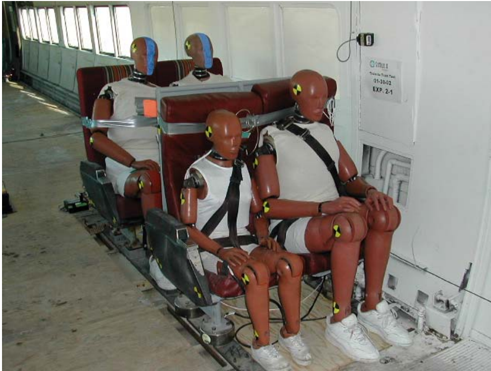
Figure 19. Pre-Test Photo of Experiment No. 2-1, Row-to-Row Intercity Seats with Front-Row Restraints
