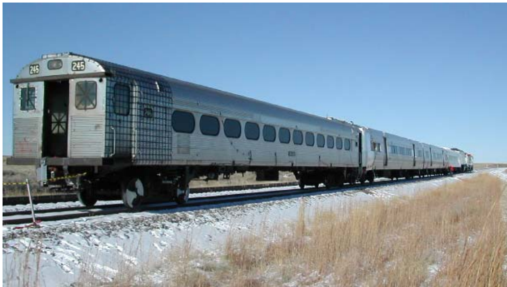
Figure 9. The Cab-Car-Led Consist with Three Trailing Coach Cars and a Locomotive
