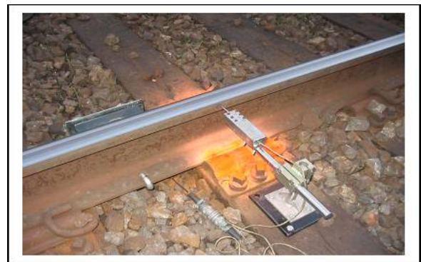
Figure 7. An LVDT based Rail Deflection Gauge (RDG) used to measure lateral rail deflections.
