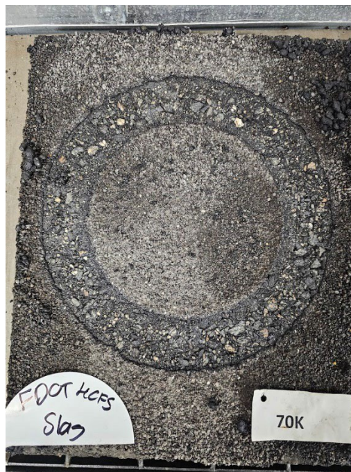
Figure 23: Failed HFCS Slab with Slag Aggregate
