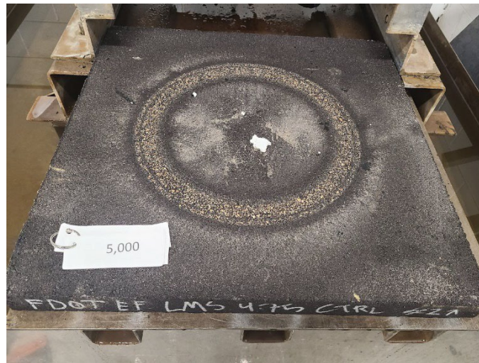
Figure 35: Initial Raveling of LMS FC-4.75 Slab at 5,000 TWPD Cycles
