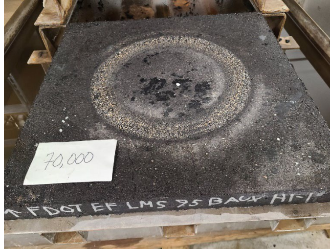
Figure 38: Raveling of LMS FC-9.5 Bauxite (High) Slab
