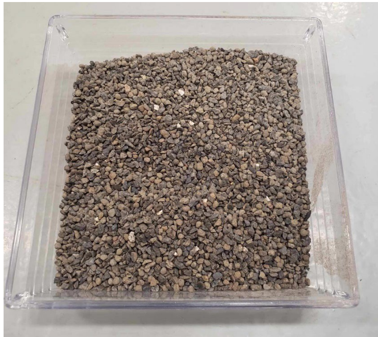
Figure 8: Sample of Calcined Bauxite from Eufala, Alabama
