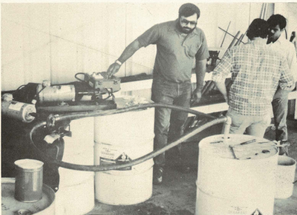
Figure 6. The resin pump was calibrated to deliver the specified amount.
