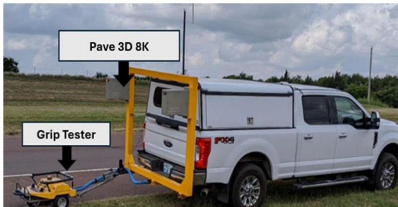
Figure 5 Pavement Friction Data Collection using Grip Tester
