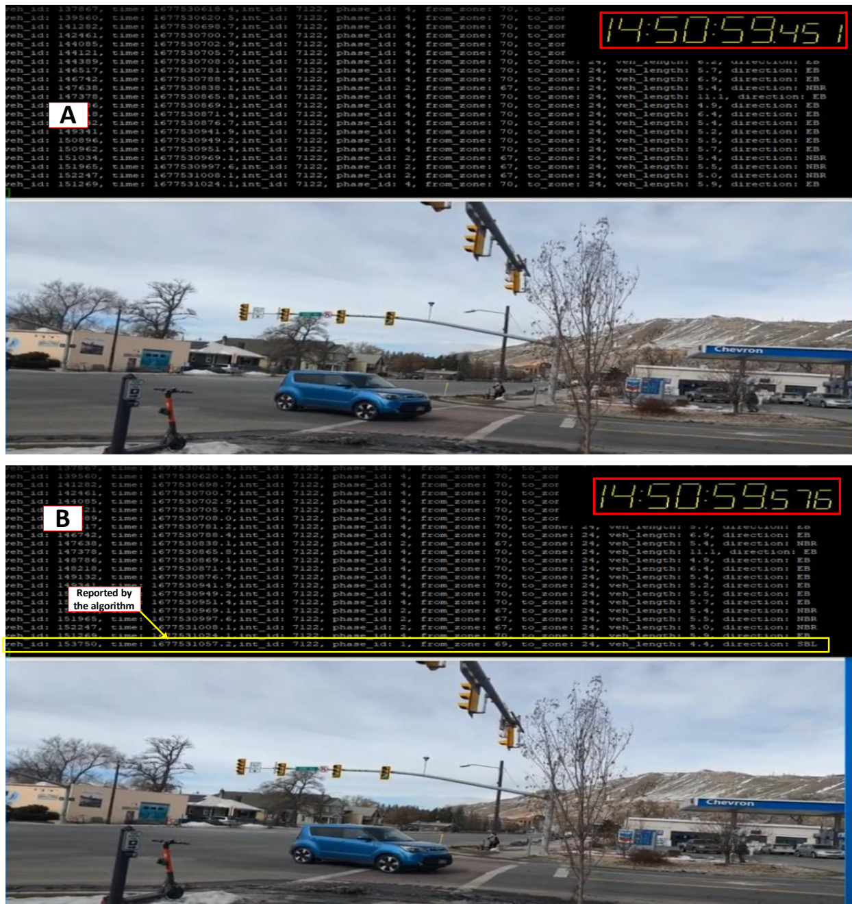
Figure 4-4 Demonstration of computing latency calculation for zone-based near-miss identification
