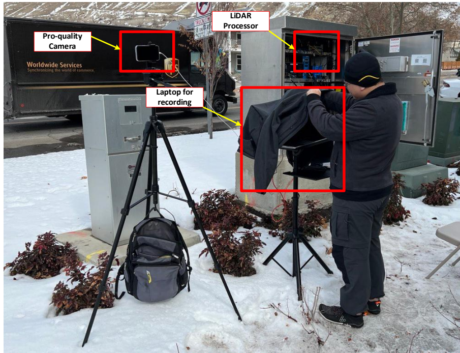
Figure 4-3 Configuration of raw data collection system
