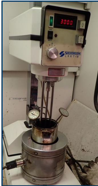
Figure 4.3 High shear mixer utilized for wet process mixing of PCR plastics into asphalt binder
