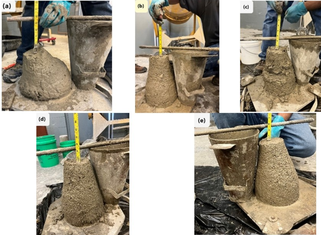
Figure 5.3 Slump-cone test (a) control (b) virgin plastic fiber (c) recycled plastic fiber-1 (d) recycled plastic fiber-2 (e) recycled plastic sand
