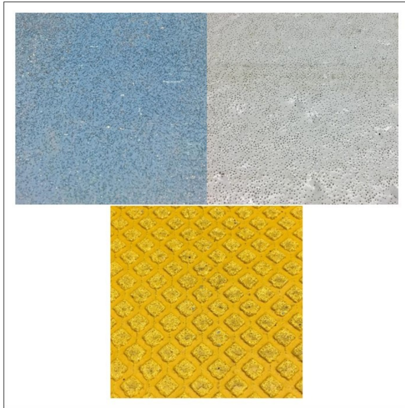
Figure 2.4 Slab surface markings for a) paint with beads, b) thermoplastic with beads, and c) cold-applied preformed tape (Nassiri, 2018)
