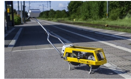
Figure 4.3 Sarsys-ASFT T2Go friction tester
