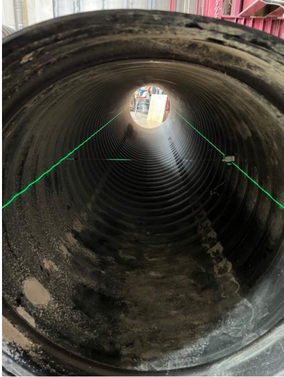
Figure 2.6 Using lasers to align instrumentation
