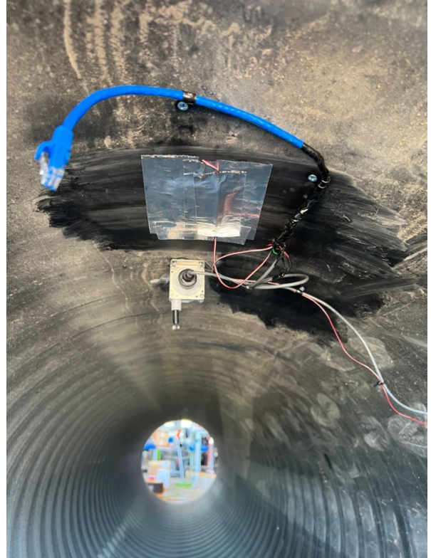
Figure 2.5 Vertical strain gauge on crown of recycled pipe (SG1-R)
