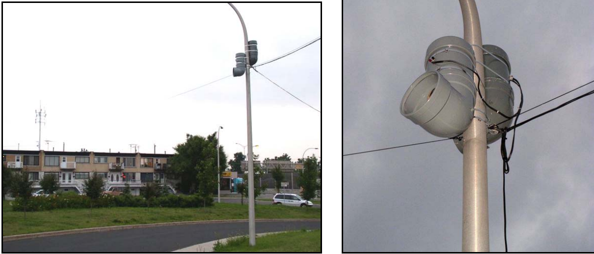
Figure 7.35 Experimental sound system used to mask nighttime construction noise in the community (Photos #42 & #38)
