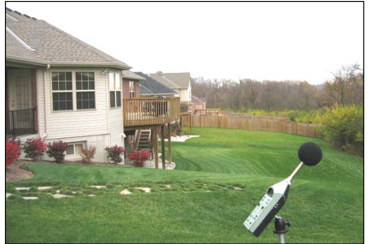
Figure 5.2 Measuring ambient noise levels in the absence of construction activity (Photo #1291)
