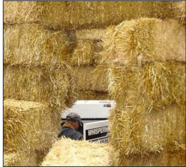
Figure 7.20 Straw bail enclosure for stationary equipment (Photo #58)
