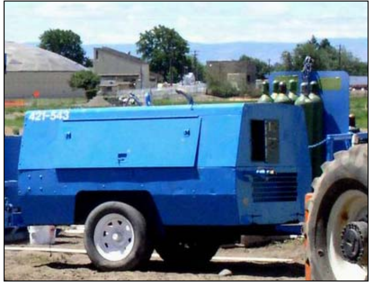
Figure 7.9 Diesel compressor with baffled housing (Photo #69)
