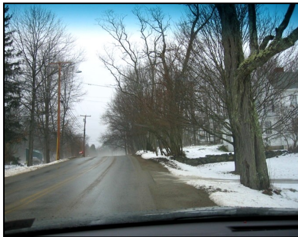
Figure 5.16 Wet roadways preclude valid noise measurements. Snow cover normally precludes valid measurements, except if a typical condition (Photo #1299)
