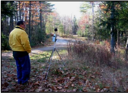
Figure 5.1 Measuring existing noise levels (Photo #1301)
