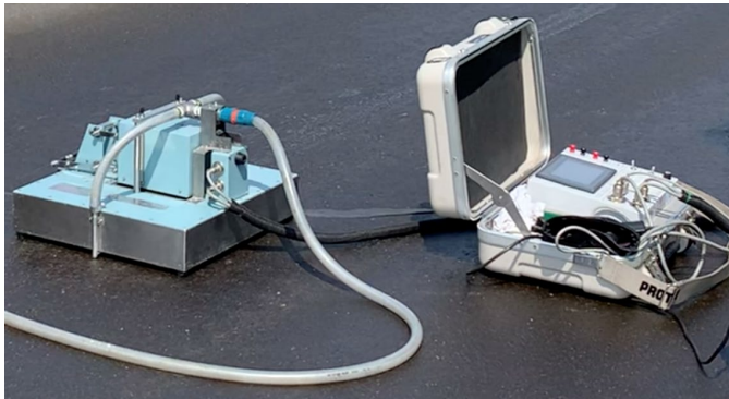
Figure 4.12 Dynamic Friction Testing (DFT) Machine used in the field measure
