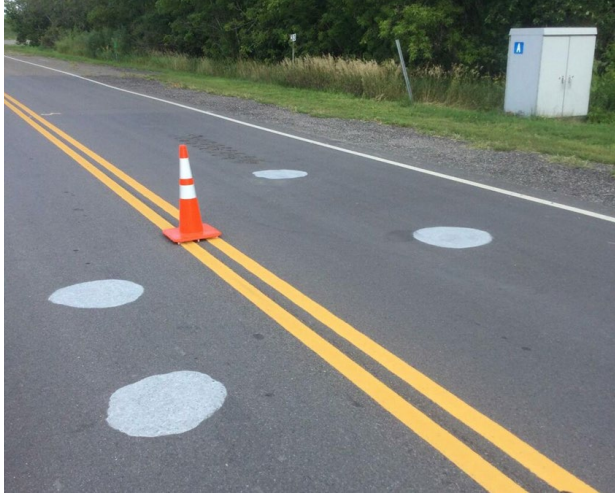
Figure 4.7 Photograph of sand patch testing in the field
