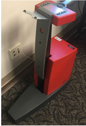
Figure 4.3 Photograph of Delta LTL-X portable retro reflectometer
