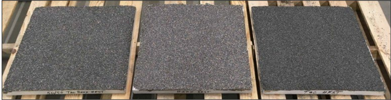
Figure D.1. Test slabs with HFST application
