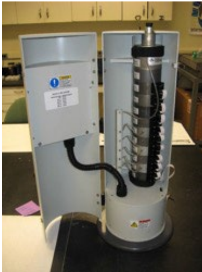
Figure 6.7. Micro-Orifice Uniform Deposit Impactor (MOUDI) (from: Monson Geerts et al., 2019)
