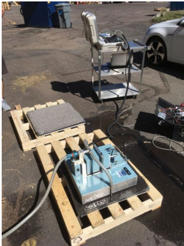
Figure 4.2. Dynamic friction tester (DFT) evaluation of simulated pavement specimens at the NRRI on June 16, 2021. Setup shows DFT, water supply hose, data interface and acquisition laptop on cart, and 12V battery for power
