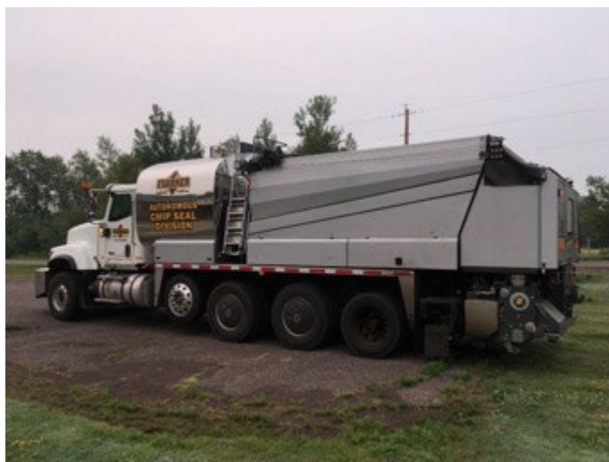
Figure 5.4. GSB Friction Seal chip spreader/distribution truck
