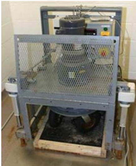
Figure D.2. Circular Track Polishing Machine (CTPM)
