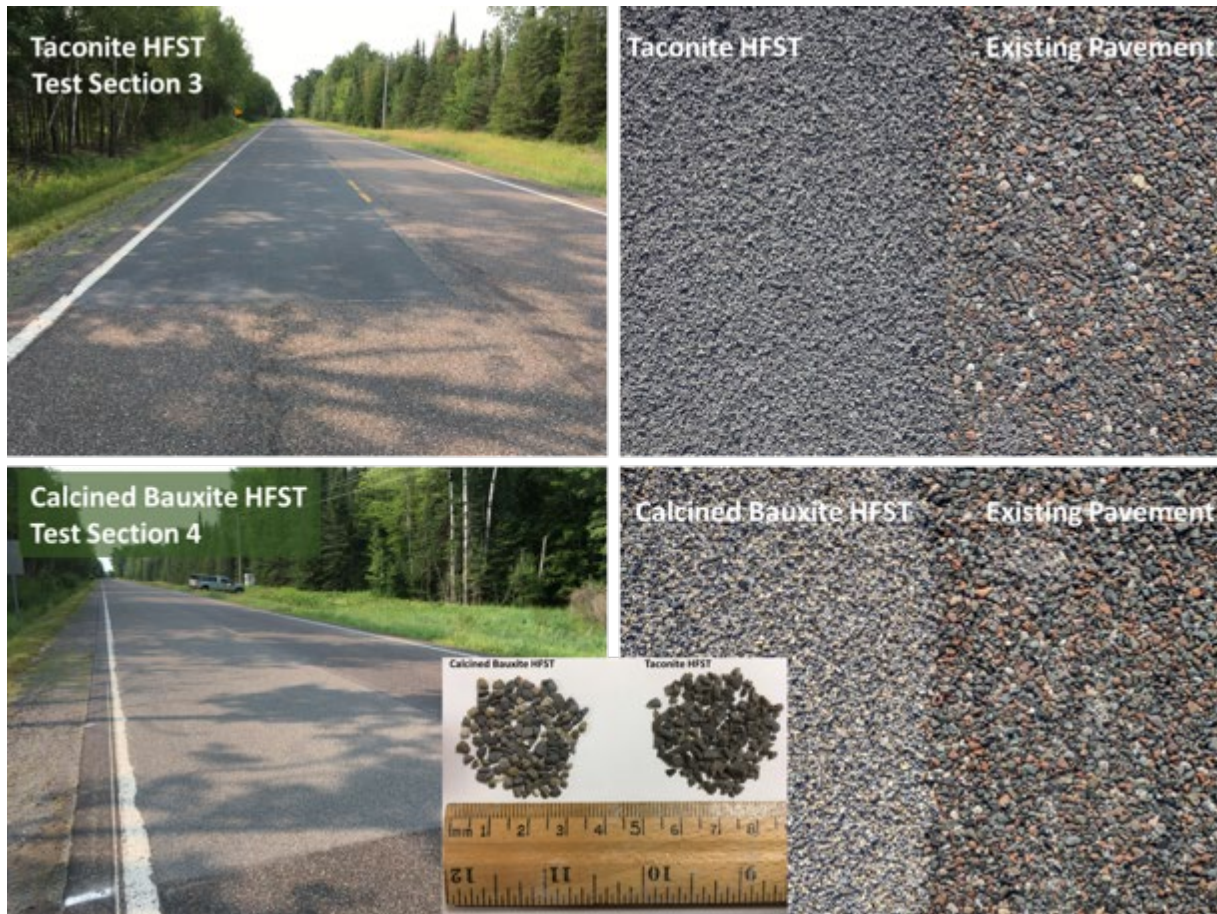
Figure 5.9. HFST test sections, post-installation: taconite test section, looking south (top left); close up of taconite HFST (top right); calcined bauxite test section, looking south (bottom left); close up of calcined bauxite HFST (bottom right); relative size of both aggregate types (inset image)
