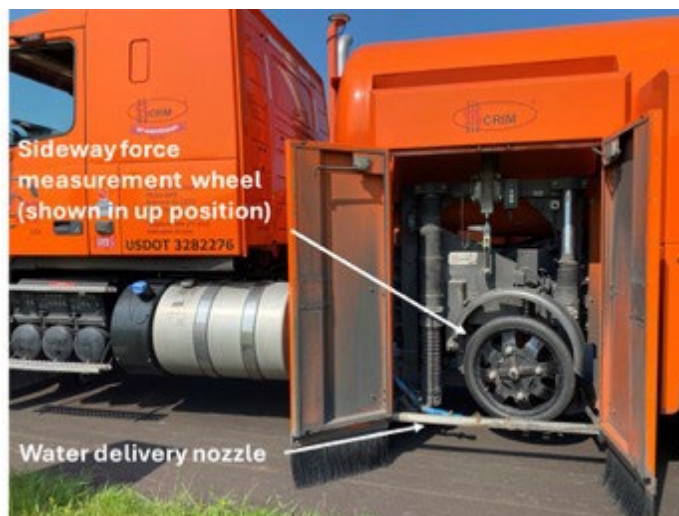
Figure 7.47. SCRIM sideway force measurement wheel and water delivery nozzle
