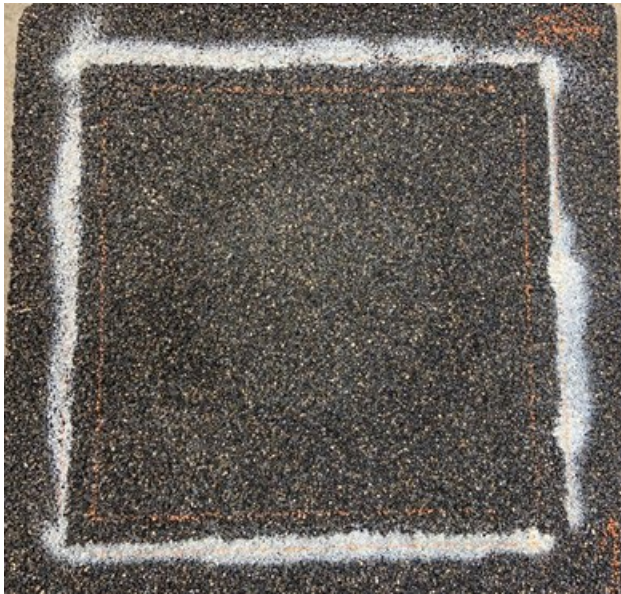
Figure D.8. 50/50 Bauxite + Taconite treatment-after testing
