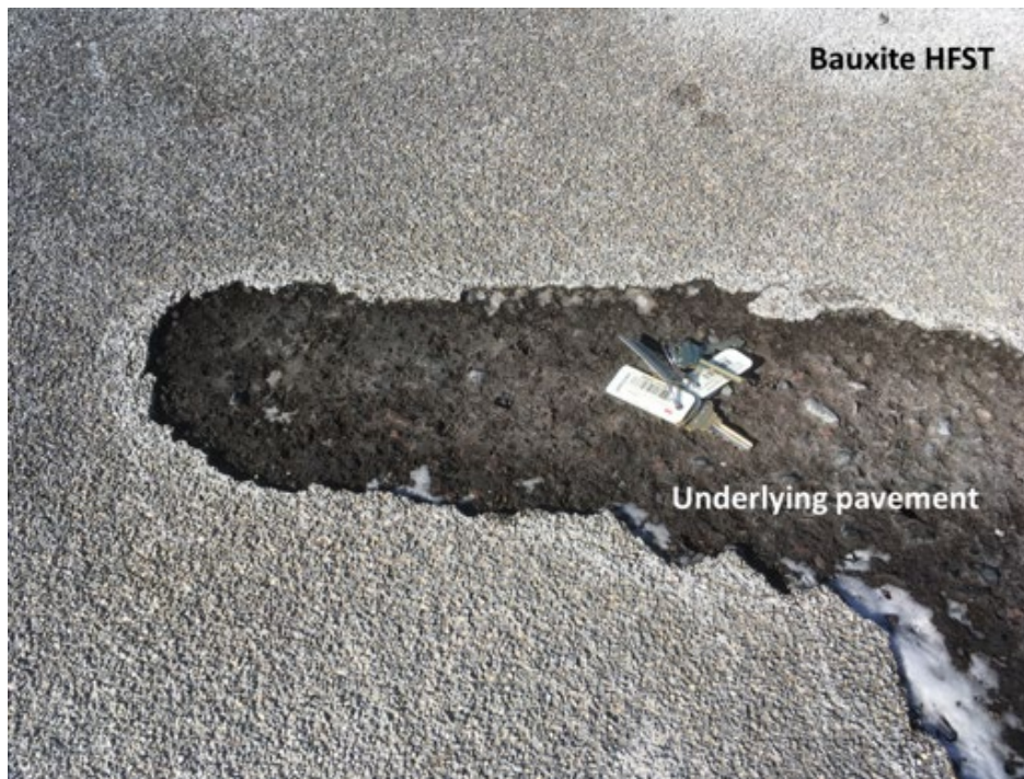
Figure 7.14. Photo showing complete exposure of underlying pavement where HFST loss occurred in the bauxite test section
