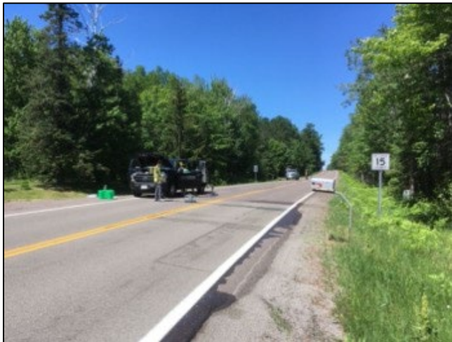
Figure 4.9. DFT and British Pendulum setup at calcined bauxite surface treatment (foreground) and existing pavement at CSAH-15 location (looking north): June 16, 2021
