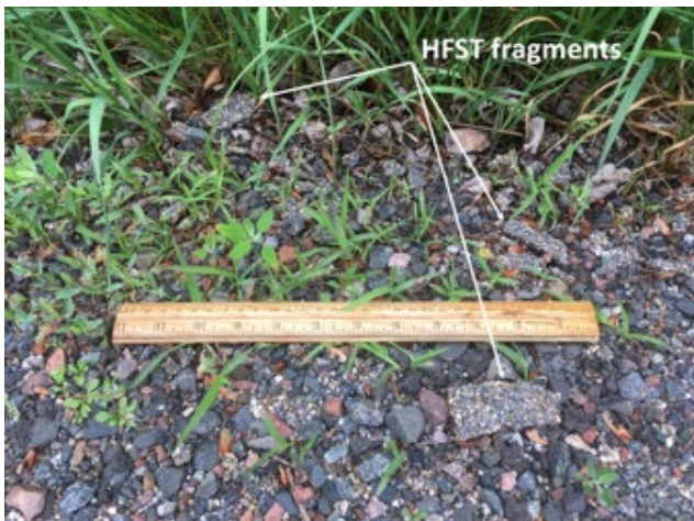
Figure 7.19. Photo of bauxite HFST fragments collected on July 5, 2022
