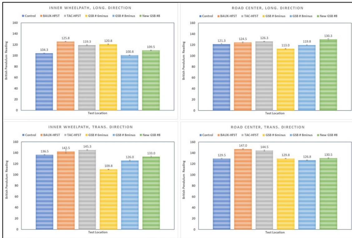
Figure 7.39. British Pendulum test results: April 30, 2024 (charts and data table)
