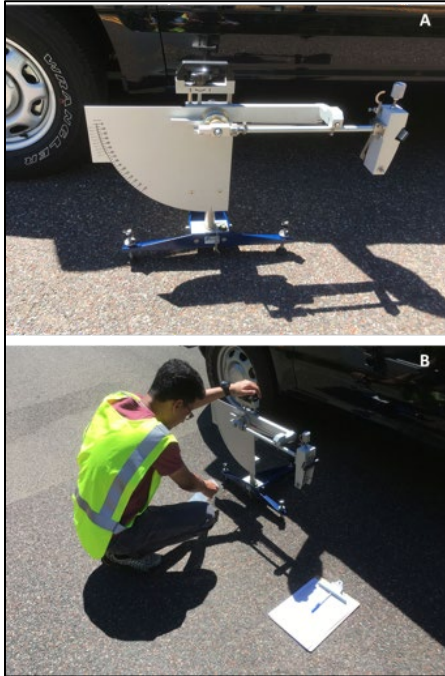
Figure 4.12. British Pendulum (A); Testing pavement friction using British Pendulum (B)
