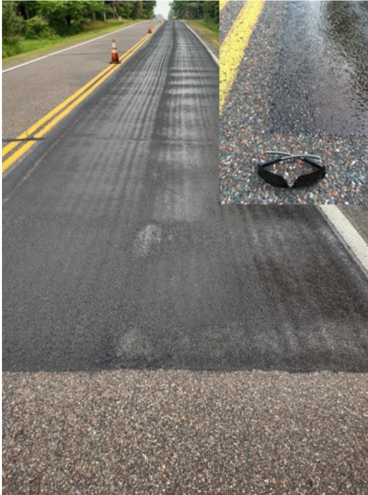
Figure 5.6. Completed Friction Seal test section and close-up image (inset)
