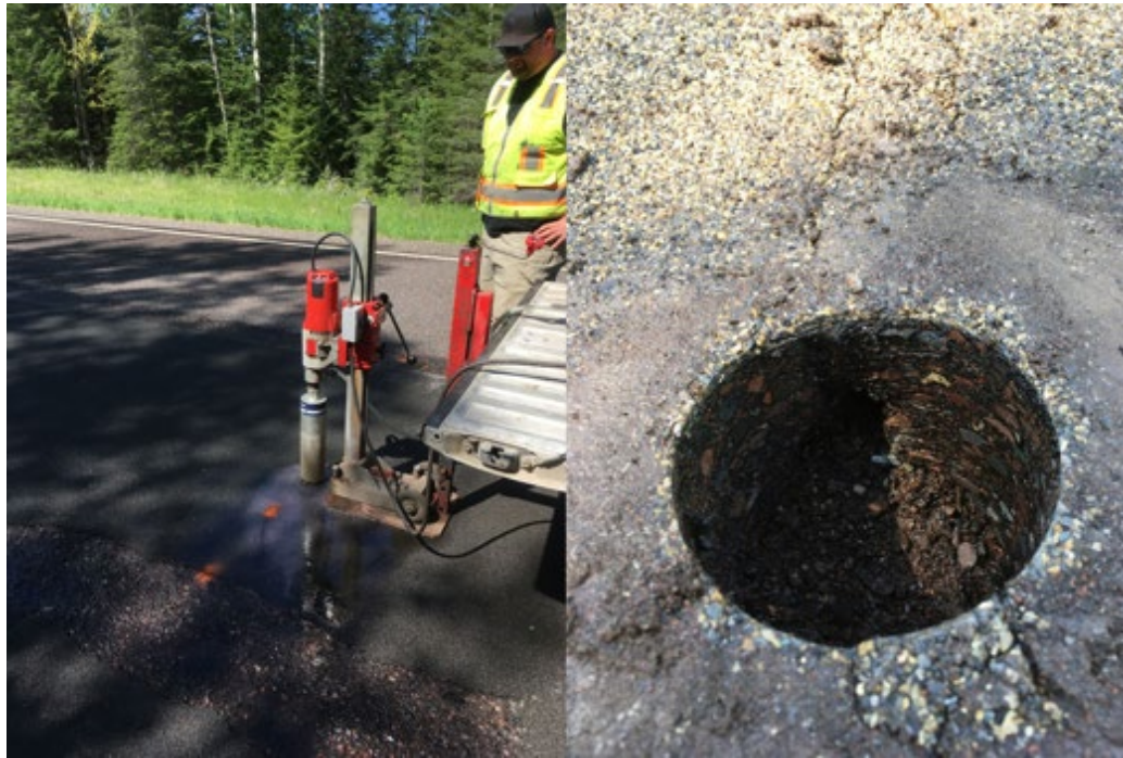
Figure 7.15. Collection of sample cores by St. Louis County personnel (left) and cored pavement (right)
