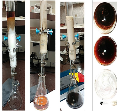
Figure 2-2 SARA fractionation test (column chromatography) (Mansourkhaki et al., 2020)
