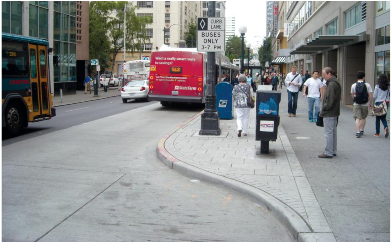
Figure 6.3 Bus Stop Curb Extension
