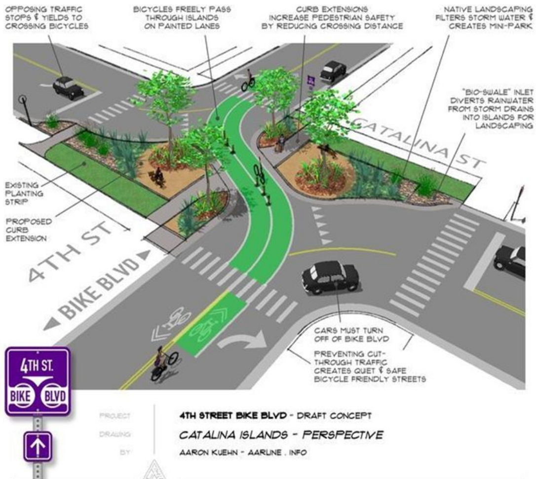
Figure 6.42 Intersection Design Featuring Vehicle Movement Restrictions
