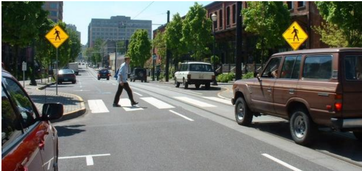
Figure 6.1 Midblock Curb Extension (also known as pinch point or choker)
