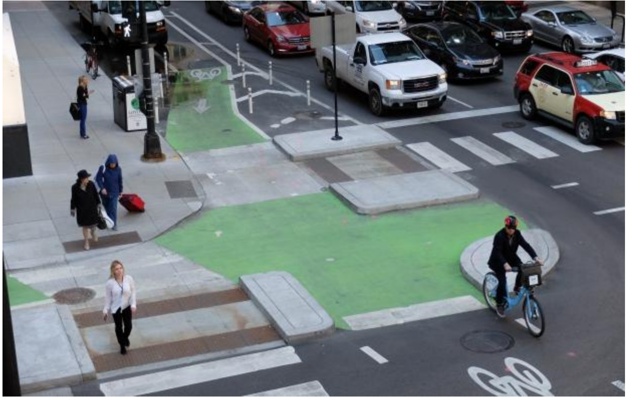
Figure 6.4 Curb Extension with Cut-Throughs for Bicyclists
