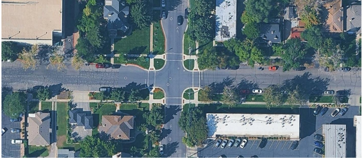
Figure 6.2 Intersection Curb Extensions (seen from an aerial perspective)
