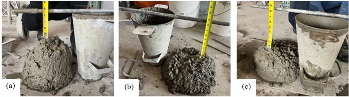
Figure 4.1. Slump test for (a) C-Q 0%, (b) C-Q 2% and (c) C-Q 4% after the addition of superplasticizer.
