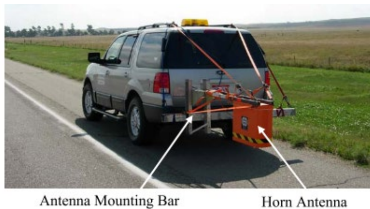
Figure 9: Horn antenna equipment field setup [4]
