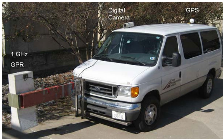
Figure 29: GPR vehicle with GPS and video camera[26]
