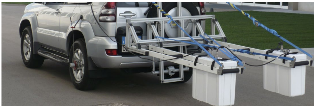
Figure 78: IDS GeoRadar RIS Hi-Pave GPR system ( idsgeoradar.com )
