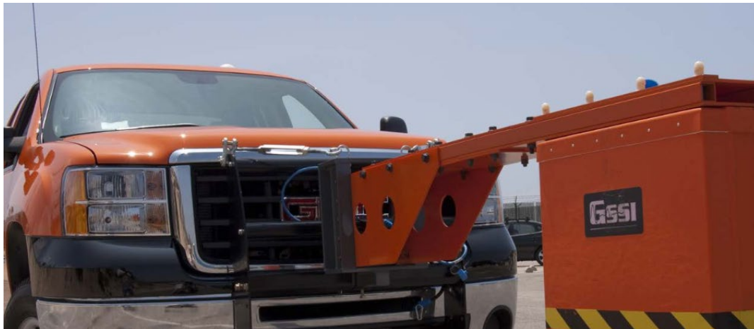
Figure 73. GSSI RoadScan 30 System with 1 Horn Antenna ( www.geophysical.com )
