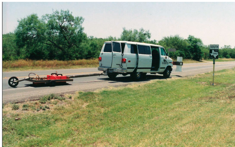
Figure 21: Combined air-launched and ground-coupled used by TTI[24]
