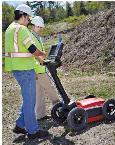
Figure 5: GPR system used for geotechnical investigation (trenchlesstechnology.com)
