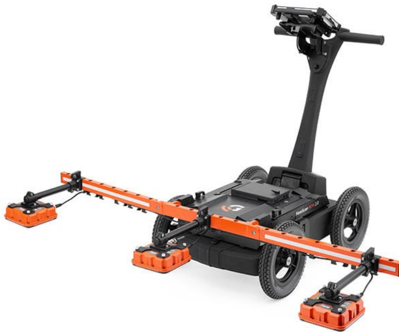
Figure 70. PaveScan RDM 2.0 with 3 Sensors ( www.geophysical.com )
