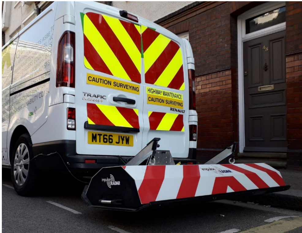
Figure 106: ImpulseRadar's Raptor GPR System ( americas.impulseradargpr.com )
