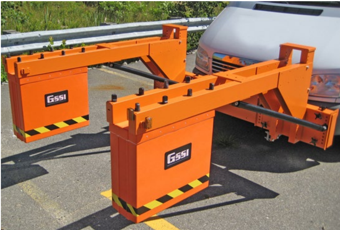
Figure 103: GSSI's RoadScan GPR system ( www.geophysical.com )
