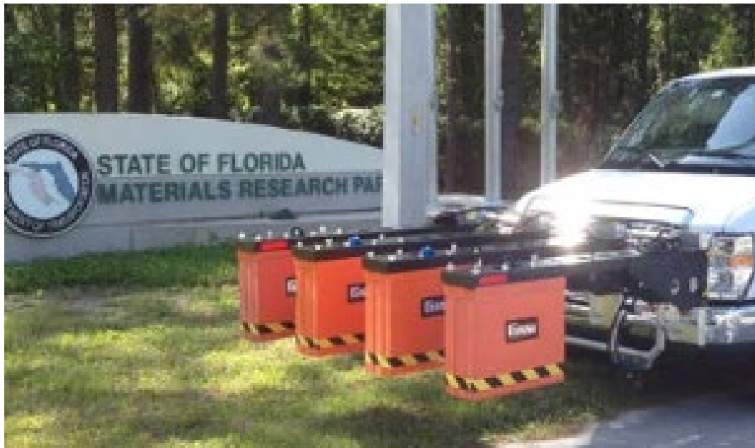
Figure 74. GSSI RoadScan 30 System using 4 Horn Antennas ( www.geophysical.com )
