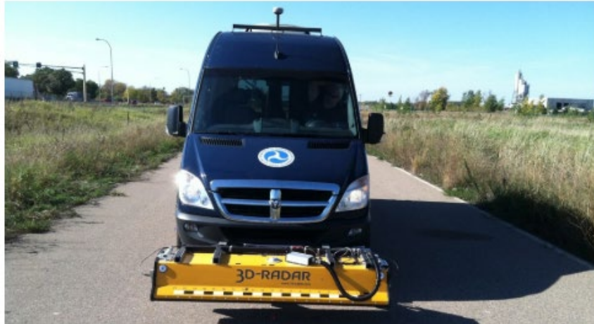
Figure 6: Vehicle mounted with 3D GPR system[19]
