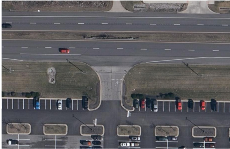
Figure 4.17 Example of an access point with a continuous median (IndianaMap, 2024).
