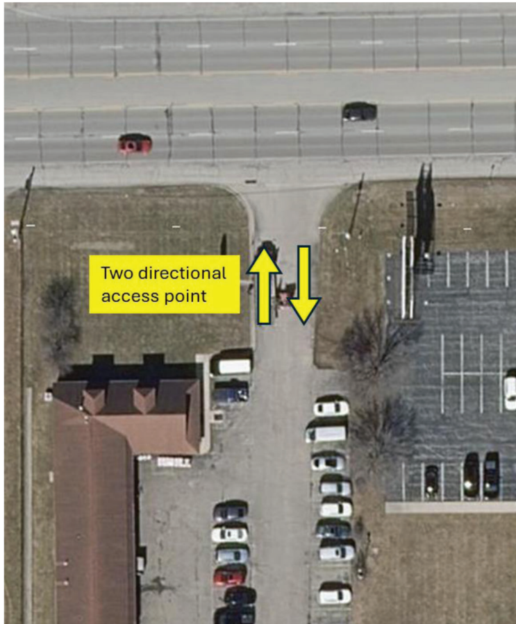
Figure 4.15 Example of a two-directional access point (IndianaMap, 2024).
