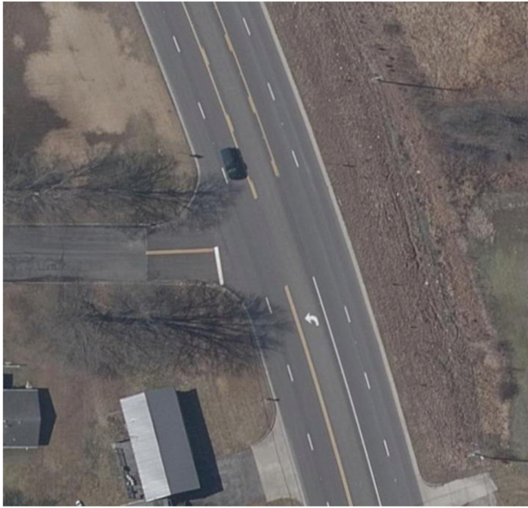
Figure 4.19 Example of an access point with unmarked pavement (IndianaMap, 2024).
