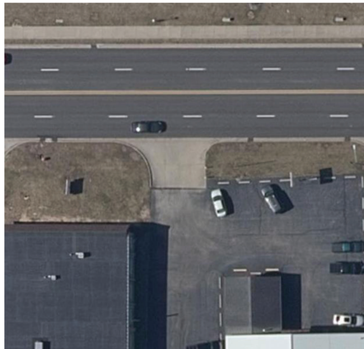
Figure 4.18 Example of an access point with a continuous centerline (IndianaMap, 2024).
