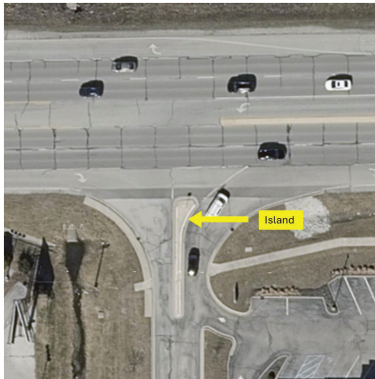
Figure 4.16 Example of a two-directional access point with island (IndianaMap, 2024).
