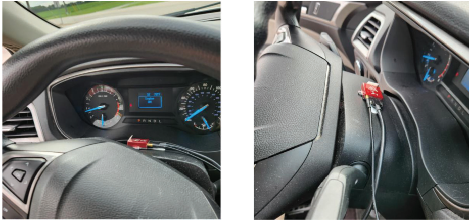
Figure 4.2 VN200 INS sensor mounted on the steering column.
